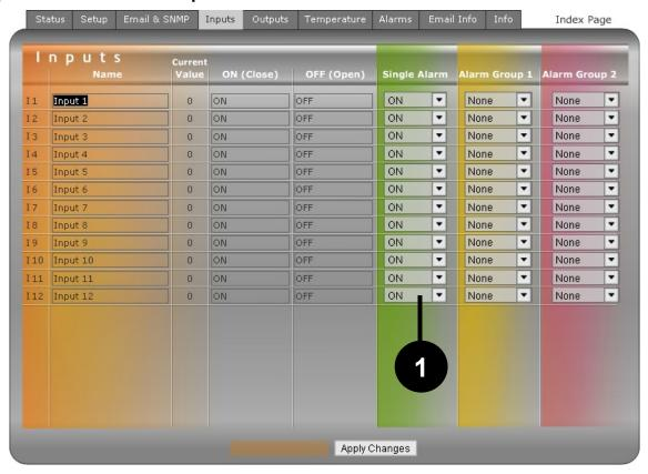
Alarm state (On or Off) to be signaled by sending an e-mail or SNMP Trap can be configured for each individual input. >> <u>Inputs</u> tab, green <u>Single Alarm</u> column.
