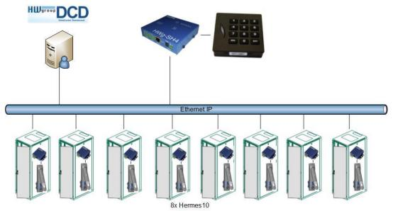
SH4 works as an RFID terminal. Door opening definition - keyboard code.
