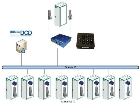
SH4 alone works as an access point. Door opening definition - keyboard code.
